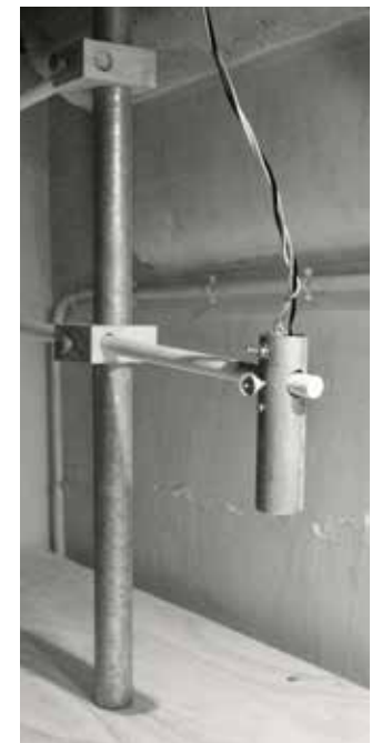
Adjustable workshop lamp, made from a scaffolding pipe, found wood and procured wiring.
